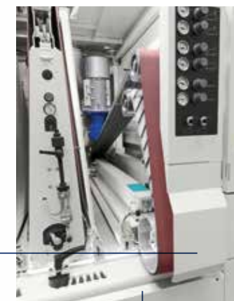
Internal crossbelt unit with 5000 mm belt length.
