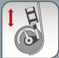
On-off pneumatic selector for rollers
