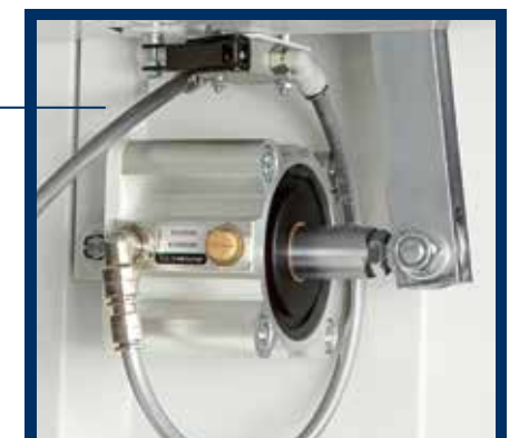
Automatic feed belt centering for a longer lifespan of the belt.
