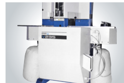
Set of two dust collecting units. Dust chute 80 mm. Air speed 20 m/sec. Air volume 320 cu.m. each unit
