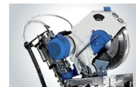
Oil-pneumatic feed of head
