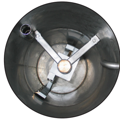
Internal scraper with blades for powder residue discharge
