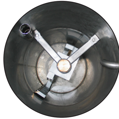
Internal shaft with scraping blades for dry residue unloading.
